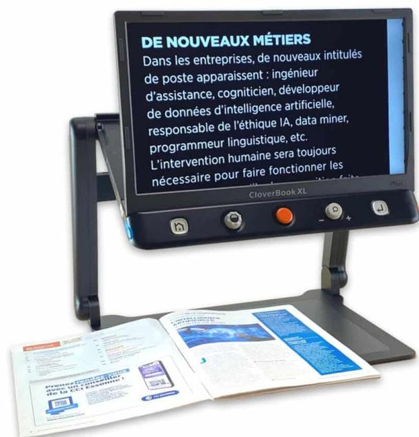
A LA FOIS UNE MAXI LOUPE ÉLECTRONIQUE ET UN MINI TÉLÉAGRANDISSEUR AVEC UN ÉCRAN DE 15,6" SOIT 40 CM. ELLE EST PLIABLE ET TRANSPORTABLE DE PIÈCES EN PIÈCES.
